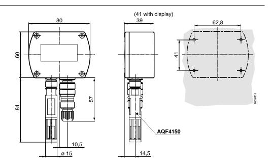
Dimensioning without (with) LCD-display
